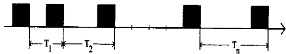
Figure 2.3: Aperiodic stream, i.e., the sequence of time intervals is neither strongly nor weakly periodic.
