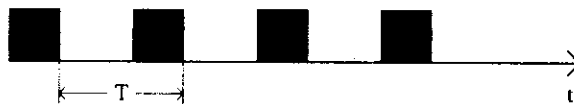
Figure 2.1: Strongly periodic stream, ( T -time limit between two consecutive packets), i.e., time intervals are of the same length between two consecutive packets.
